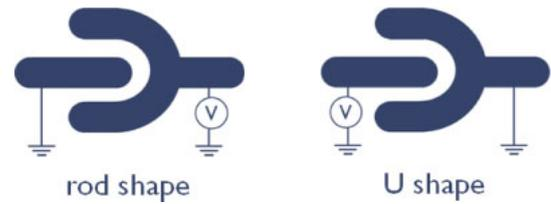
**Fig. 6.** (Color online) Conceptual configurations of source bias conditions for half-Corbino a-Si:H TFTs.
