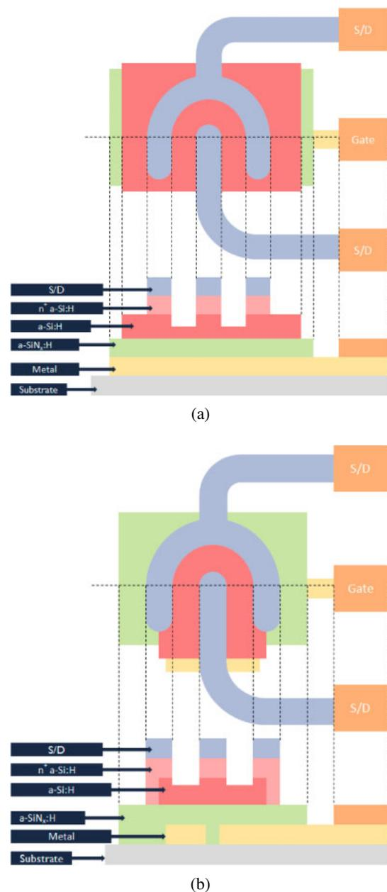
Fig. 2. (Color online) Cross-sectional views of half Corbino TFT with (a) unpatterned gate electrode and (b) patterned gate electrode.
