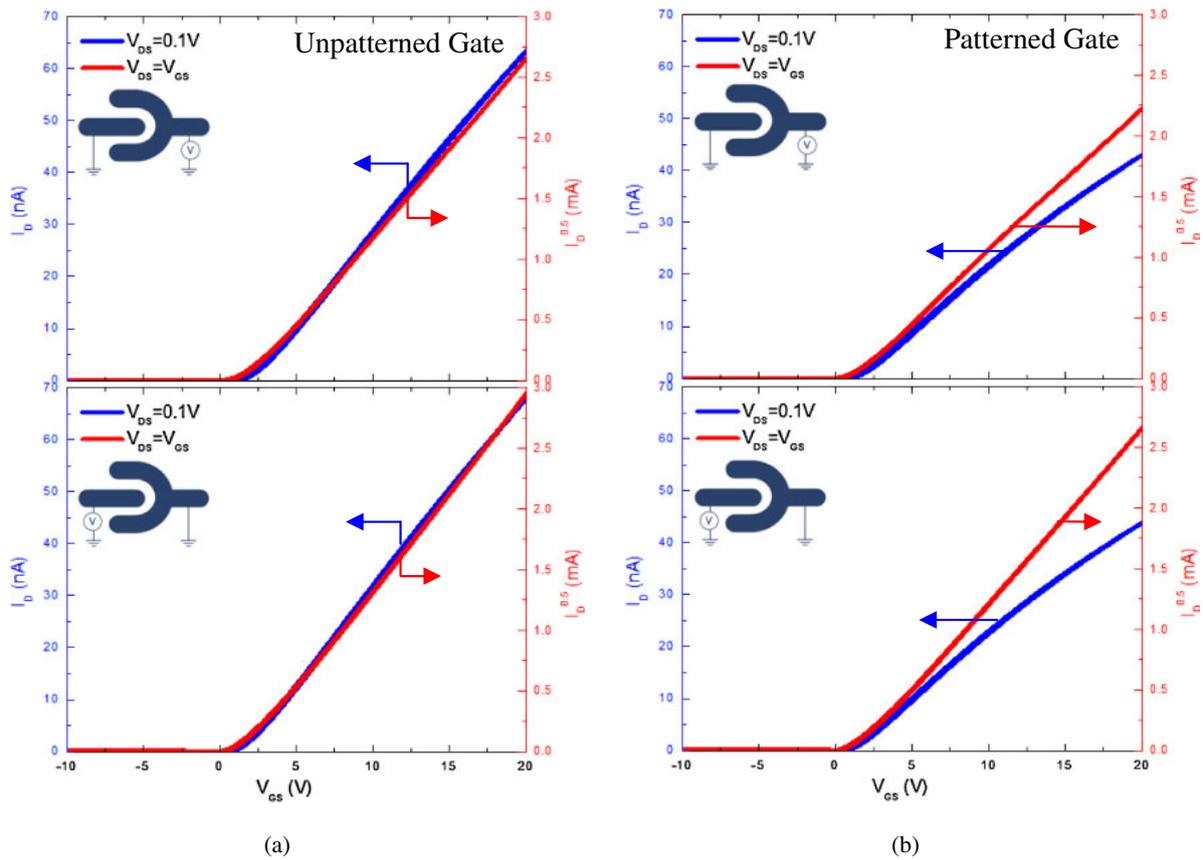
**Fig. 7.** (Color online) Asymmetric transfer characteristics of half Corbino a-Si:H TFT with  $L = 6 \mu\text{m}$  and  $OV = 6 \mu\text{m}$ . Curves used for extraction of the threshold voltage and mobility are also shown: (a) unpatterned gate electrode and (b) patterned gate electrode.
