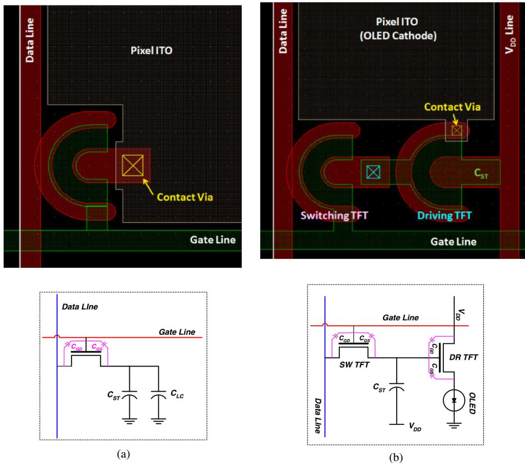
**Fig. 8.** (Color online) Top views and their equivalent circuits of the proposed half-Corbino a-Si:H TFT pixel circuits for (a) AM-LCD and (b) AM-OLED.
