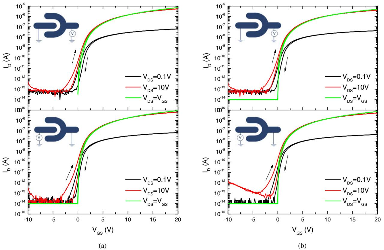
**Fig. 4.** (Color online) Asymmetric transfer characteristics of half Corbino a-Si:H TFT with  $L = 6\ \mu\text{m}$  and  $OV = 6\ \mu\text{m}$  for different source bias conditions: (a) unpatterned gate electrode and (b) patterned gate electrode.
