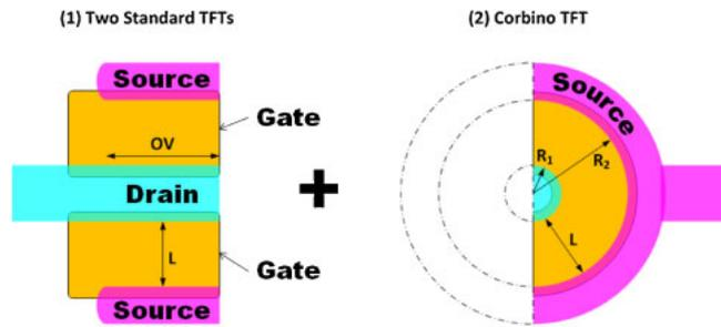
**Fig. 5.** (Color online) Conceptual configuration of effective channel width and length (geometric factor) definition for half-Corbino a-Si:H TFT.
