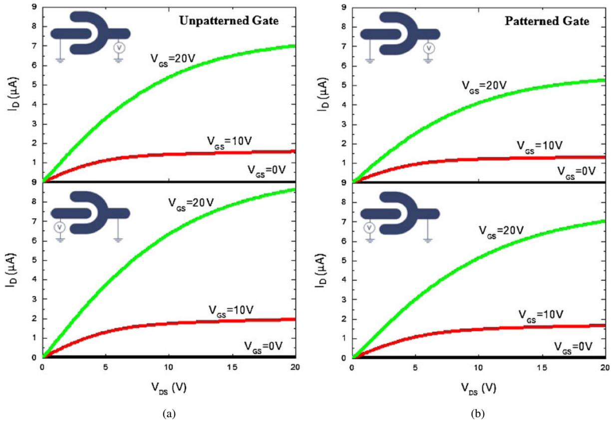
**Fig. 3.** (Color online) Asymmetric output characteristics of half Corbino a-Si:H TFTs with  $L = 6\ \mu\text{m}$  and  $OV = 6\ \mu\text{m}$  for different source bias conditions: (a) unpatterned gate electrode and (b) patterned gate electrode.
